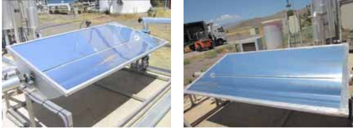
Figure 2. CAPSOL prototypes installed at the PSA: CAPSOL-01 (left) and CAPSOL-02 (right)
