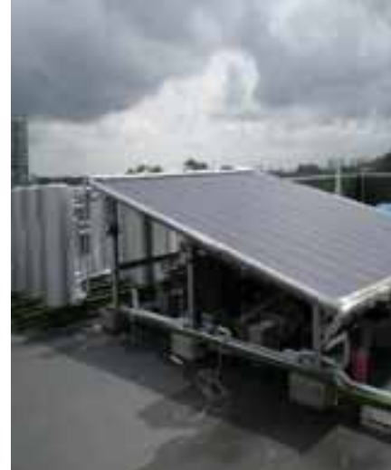
Fig. 5: Structure and photo of 1.532kW p a-Si forced circulating PVT system
