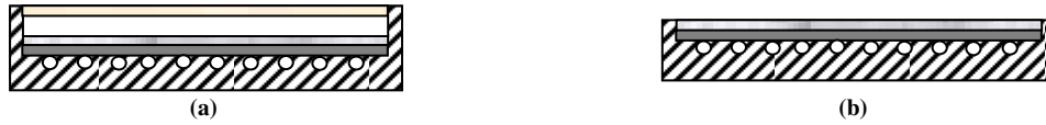
Fig. 1: sectional view of (a). a glazed PVT collector and (b). an unglazed PVT collector
