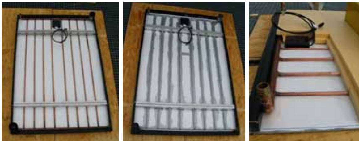
Fig. 2: Pipe heat exchanger glued to PV module without insulation (epoxy, epoxy-AL) and with insulation (epoxy)
