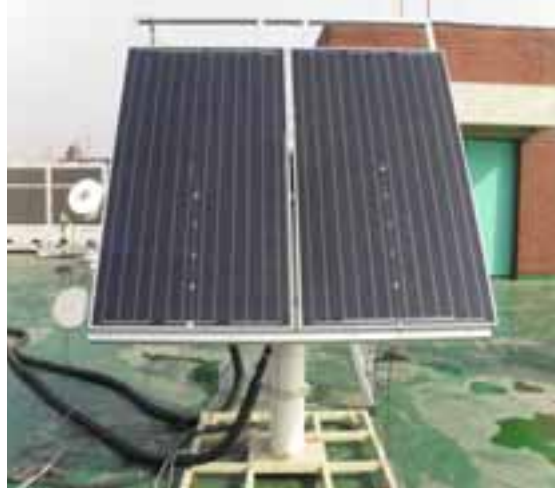
Fig. 3: Experiment view of sheet-and-tube and fully wetted absorber PVT collector
