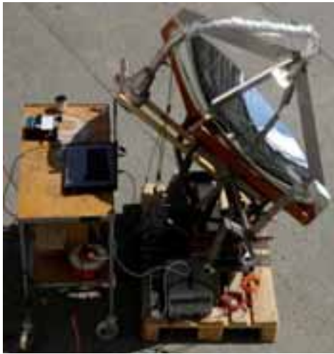
Fig.1: Test rig for absorbers experiment, a Photograph (left) and schematic drawing showing the location of the thermocouples (right)
