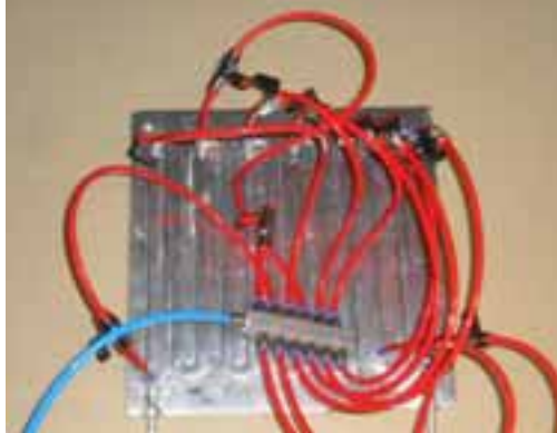
Fig. 14: Sample meander panel with a number of pressure measuring points
