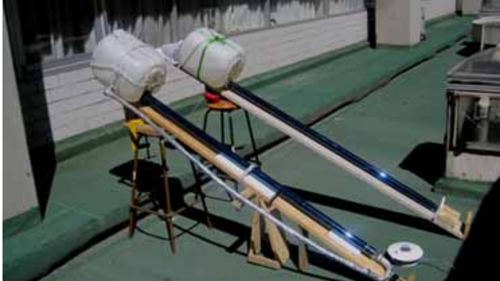
Fig. 1. Photo of the solar collector experimental set up, one system with a water storage and a solar absorber tube with a recirculation tube, one entrance and one water exit. The other system equivalent to the first one, but the solar absorber tube without a recirculation tube, one end closed.
