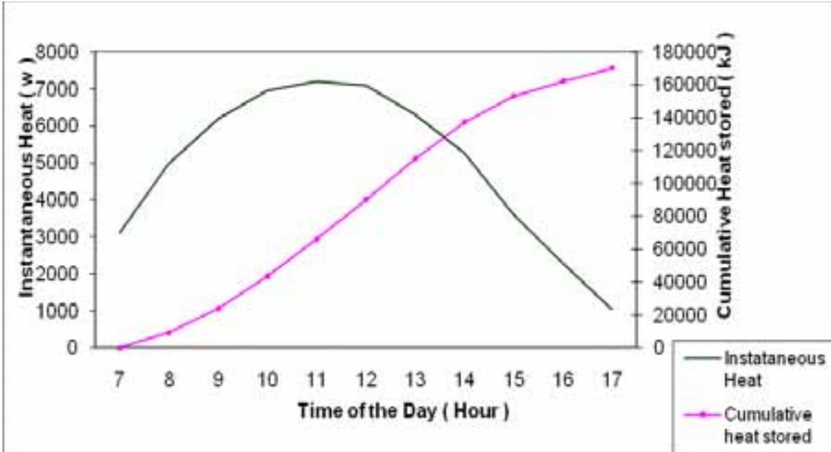
Figure 4. Variation of Instantaneous and cumulative energy stored with time during the month of March ( m = 2 \text{ kg/min} )
