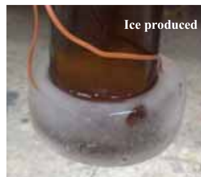
Fig. 4: Two photographs of the solar ice maker and ice produced
