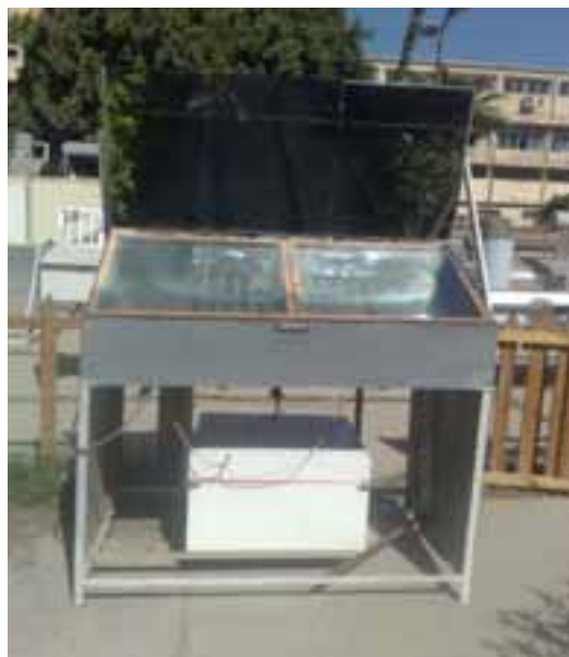
Fig. 4: Two photographs of the solar ice maker and ice produced
