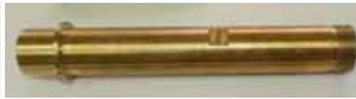
Fig. 17: Photograph of the tested mixing chamber
