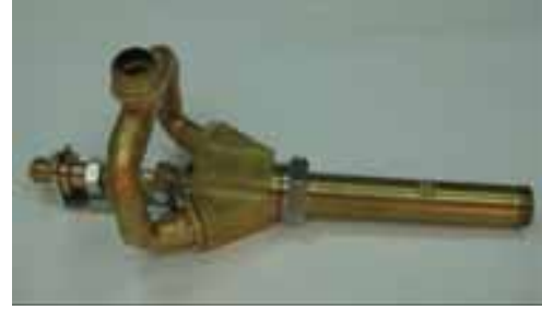
Fig. 15: Photograph of the ejector assembly
