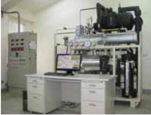
Fig. 14: Photograph of the ejector test rig
