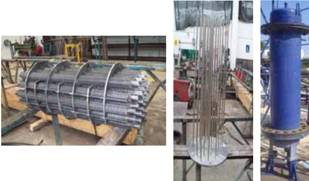
Figure 3 Pictures of the thermo-chemical reactor (STIR): a) tube and shell heat exchanger; b) gas refrigerant (NH 3 ) distributors; c) complete thermo-chemical reactor
