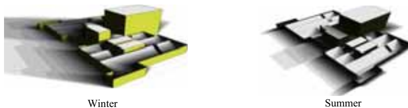
Fig. 3: Shading calculation for a studied solar installation
