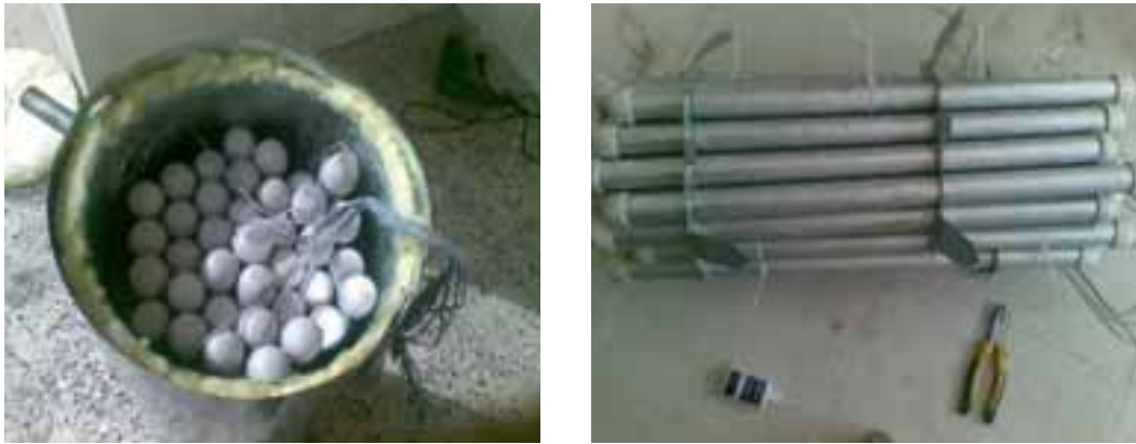
Fig. 3: PCM capsules used in the heat exchanger.
