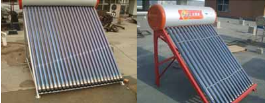
Fig. 1: Close-packed ETC (L.) and ordinary ETC (R.) used in the experiment
