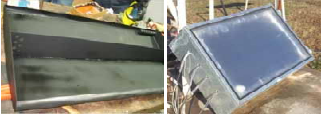
Fig. 6: The absorber-storage tank in construction and the complete system with the thermocouples connected.
