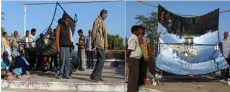
Fig. 2 Tribal workers installing PRINCE-40 concentrators and Cooking in action.
