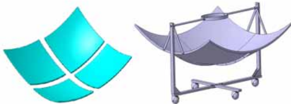
Fig. 4 Exploded view of model of segmented dish and assembly of concentrator.
