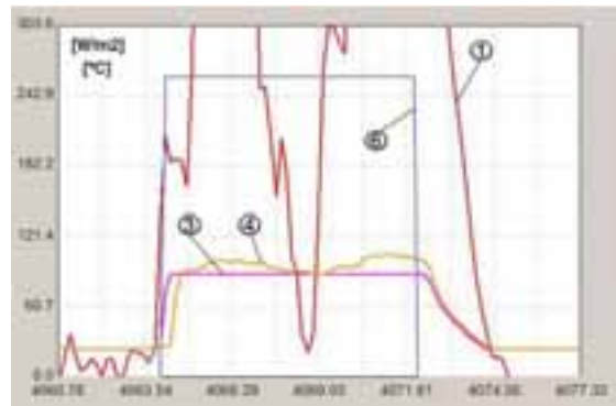
Fig. 6. DNI, P_t , T_{in} , and T_{out} in a cloudy day of June
