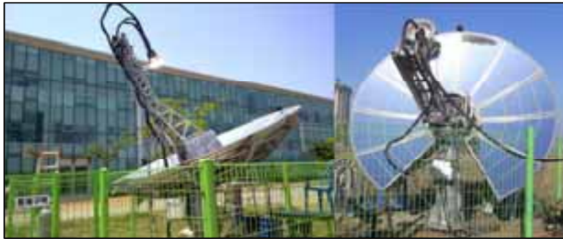
Fig. 4 Dish-type solar thermal system (Inha Dish-1)
