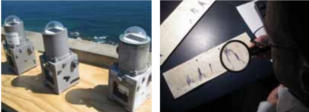
Figure 1: Actinographs of the NSA (left), and Mr. Roberto Sotta of the NSA processing results.
