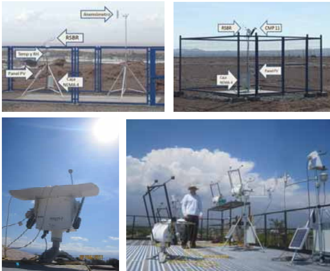
Figure 4: Two different configurations for RSBR stations (top); one BSRN-standard station (bottom left); author Alberto Ortega at the UC Solar Evaluation Lab in Santiago (bottom right) where both BSRN-standard and RSBR radiometers are tested prior to field deployment. Nice clouds over the Andes Mountains at the back.
