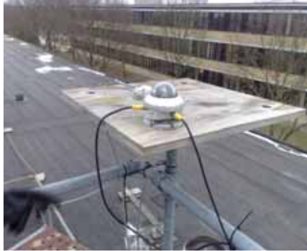
Fig. 2: Pyranometer measuring the solar radiation
