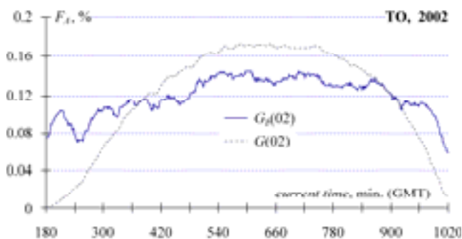
Fig. 11: Frequency of (fast)alternating clouds assessed by global radiation G(02) and its beam fraction G_b(02)
