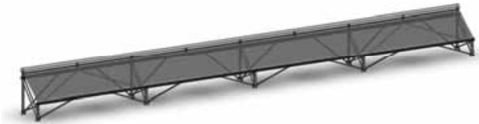
Fig. 1: SAED solar collector unit
