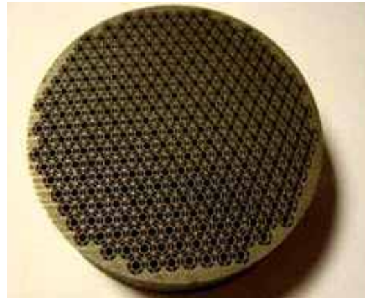
Fig. 13: Compact heat exchanger realized through SLM process
