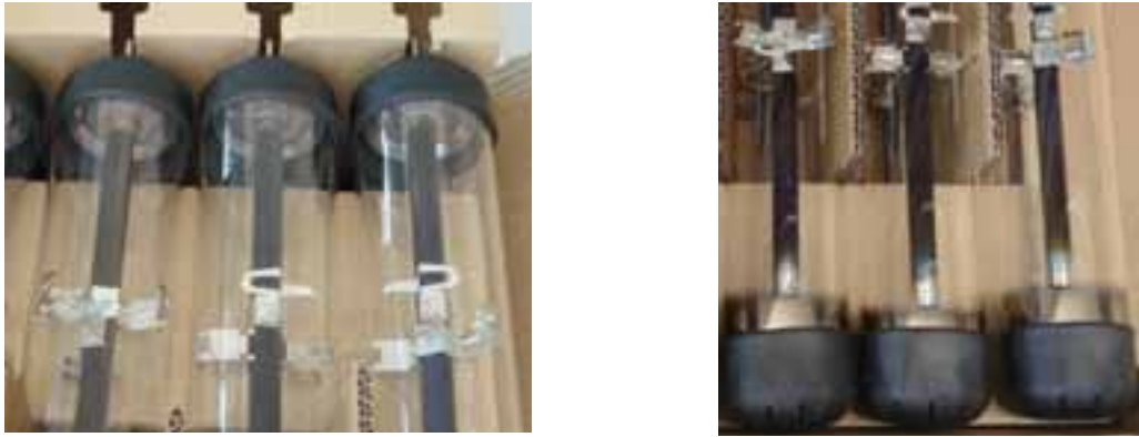
Fig. 10: Details from the first series of tube. The coating has been deposited directly on the stainless steel tube
