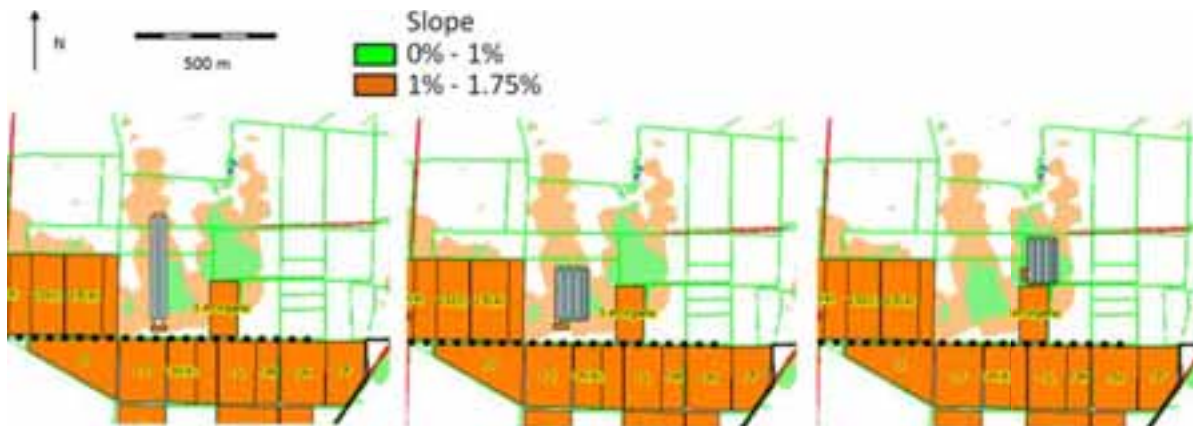
Fig. 6: Possible linear Fresnel plant setup with two lines (left) and four lines (middle and right)
