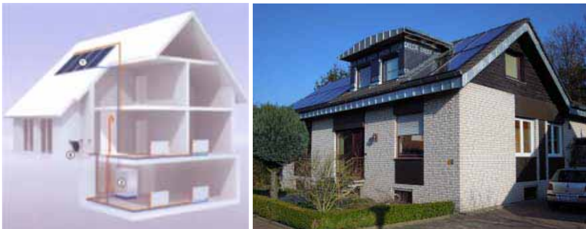
Fig. 7: Schematic view of the monitored system B, 1: solar thermal collectors, 2: hybrid heat pump, 3: external split unit
