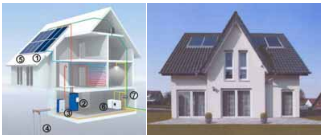
Fig. 2: Schematic view of the monitored system A, 1: solar thermal collectors, 2: solar hot water storage and solar station, 3: brine/water heat pump, 4: borehole heat exchanger, 5: PV modules, 6: power inverter, 7: electric meter [Schüco]
