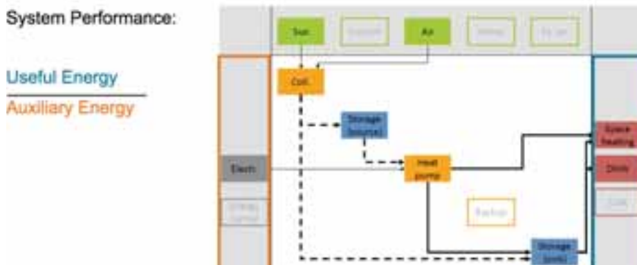
Using the square view to show one definition of the system performance (blue rectangle = the output divided by orange rectangle = the non local energy input)
