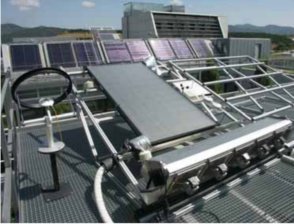
Fig. 1: Outdoor quasi-dynamic testing bench
