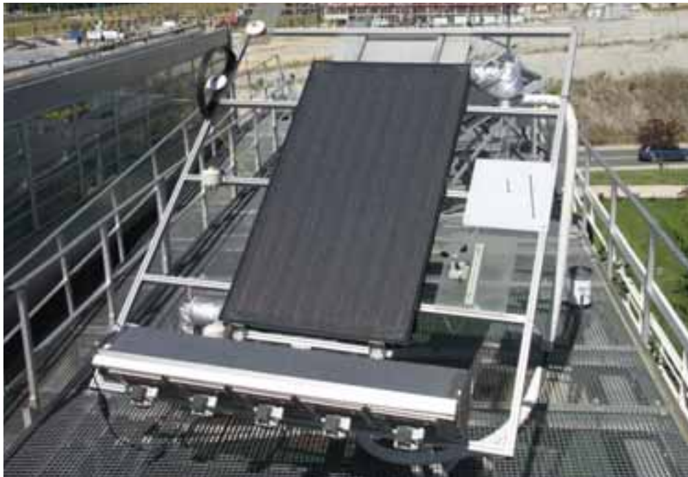
Fig. 2: Outdoor steady state test bench with solar tracker
