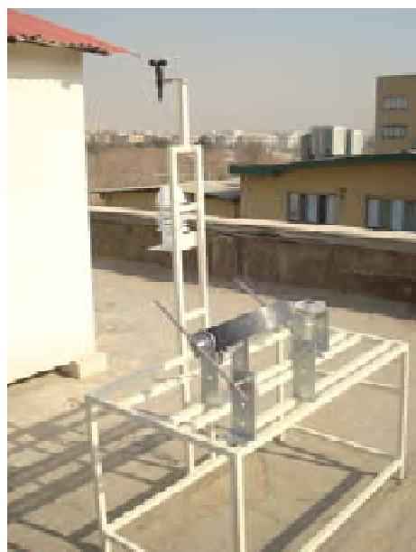
Fig. 4: Weather station including equipments for recording weather conditions at the test station
