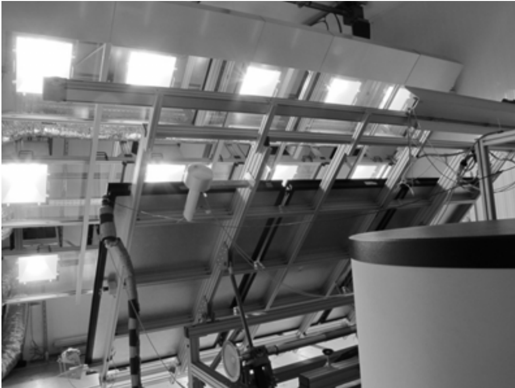
Fig. 2: View of the solar simulator. At the back: Lamp array with cold sky. In the foreground: collector support rig with three collectors and hot water store on the right
