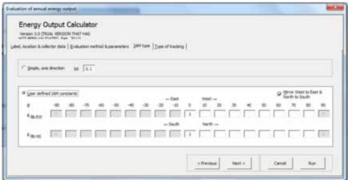
Figure 4. Step 4: Incidence angle modifier input page. Also extreme double asymmetrical collectors can be handled.
