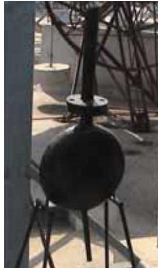
Figure 5: An example of a round flask shaped receiver used with Scheffler Reflector process heat steam systems.[Source: De Wet van Rooyen]
