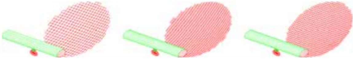
Figure 9: Scheffler Reflector with different mirror tile geometries
