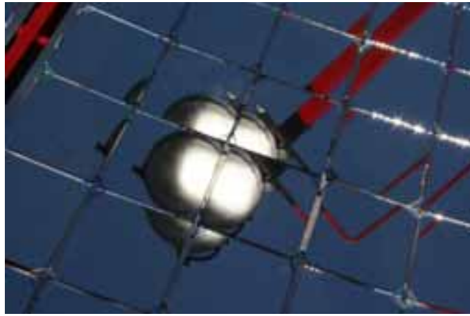
Figure 4: The focal point of a 2.7 m 2 Scheffler Reflector solar cooker is seen reflected in the mirror tile segments of its primary reflector.[Source: Denis-Luc Ardiet]
