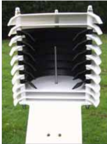
Figure 1: Cross-sectional view of a Stevenson Screen (Campbell, 2010)
