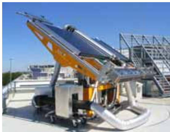
Fig. 1: Solar air heating collector installed on the outdoor test facility at Fraunhofer ISE
