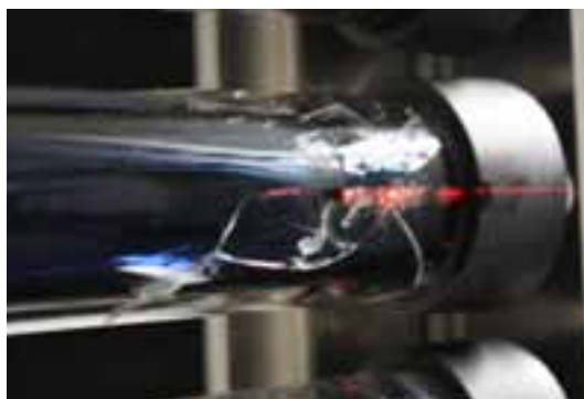
Fig. 4: Typical damage symptoms of a Sydney-pipe after shot on the clamp
