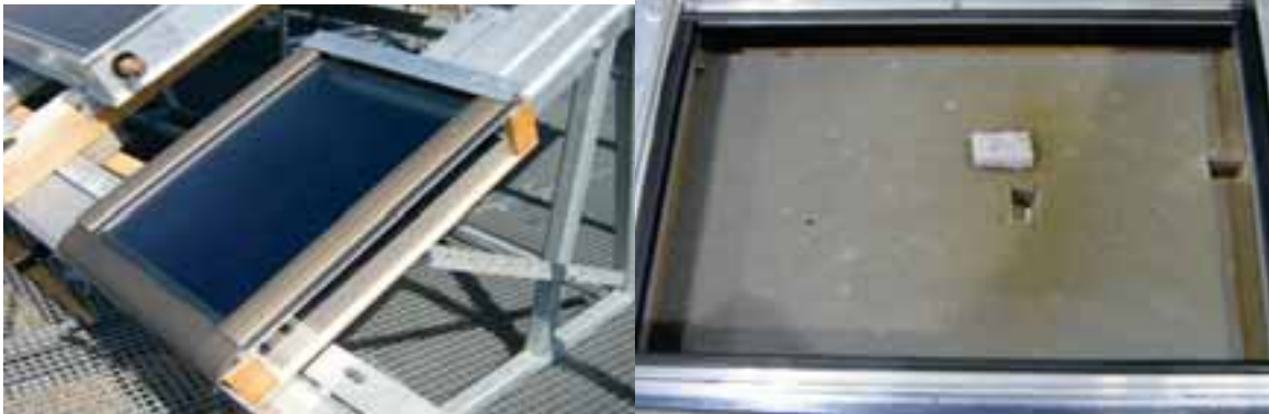
Figure 10: Miniature Collector (70x40 cm 2 ) employing a special type of soft polyurethane foam insulation. Left: Collector was exposed more than one year in Vienna. Right: yellowing of the foam below the absorber and sample for SEM and ATR-FTIR.
