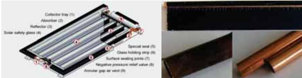
Figure 4: Left: Scheme of a CPC-collector ( www.solarfocus.at ). Right: Absorber (top) and manifold pipes (bottom left: after brazing, bottom right: new) of the CPC collector
