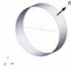
Figure 2: Discretised cylinder surface showing the normal vector n for a surface element.
