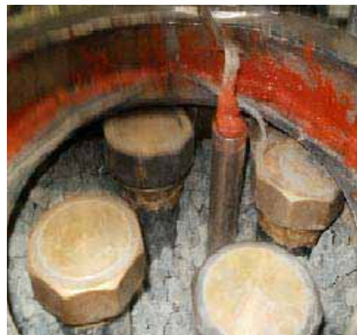
Figure 2: showing the Cu PCM cylinders with rocks for heat storage
