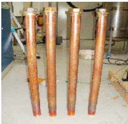
Figure 1 showing copper cylinders containing with PCM
