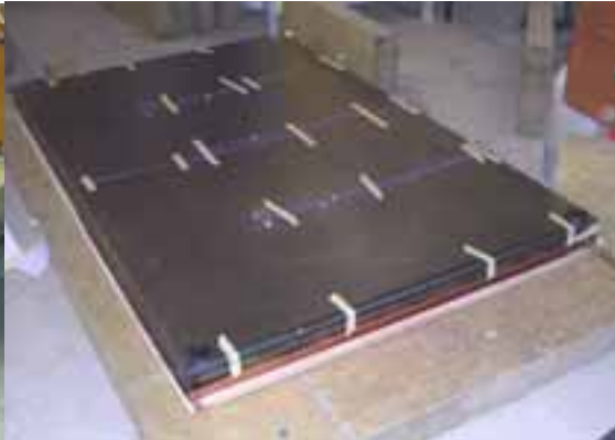
Fig. 3: Photos of the heat storage module with a copper absorber used for the heat transfer.
