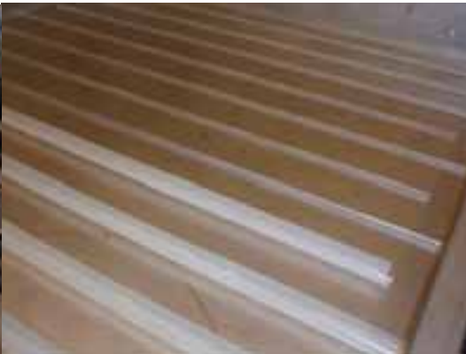
Fig. 3: Photos of the heat storage module with a copper absorber used for the heat transfer.
