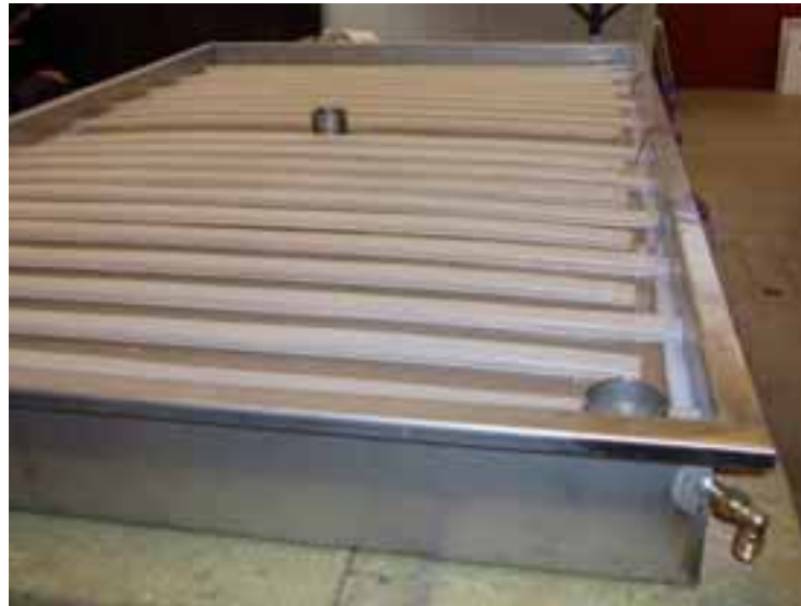
Fig. 1: Photo of the PCM heat storage test module with plate heat exchangers at the top and the bottom.
