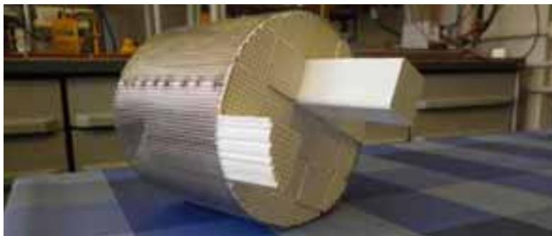
Fig. 1: Honeycomb structure of a composite storage material mullite/salt mixture for a lab-scaled open thermochemical storage
