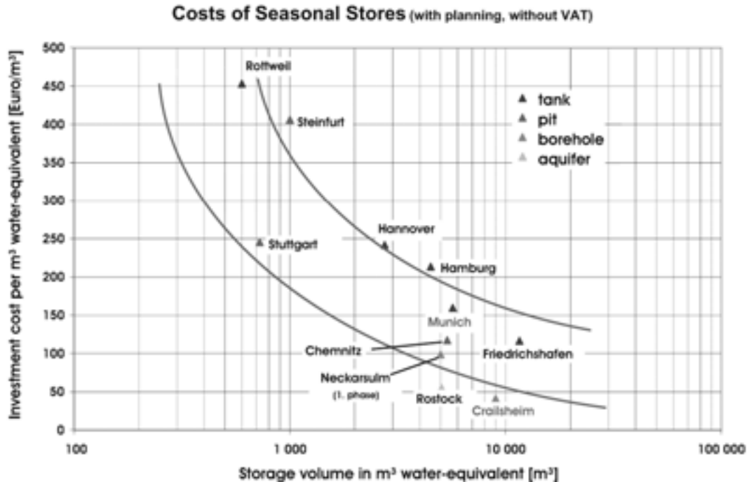
Fig. 3: Cost of seasonal stores for Central Solar Heating Plants with Seasonal Storage (Lottner et al. 2000, Schmidt et al. 2004, Mangold 2007)
