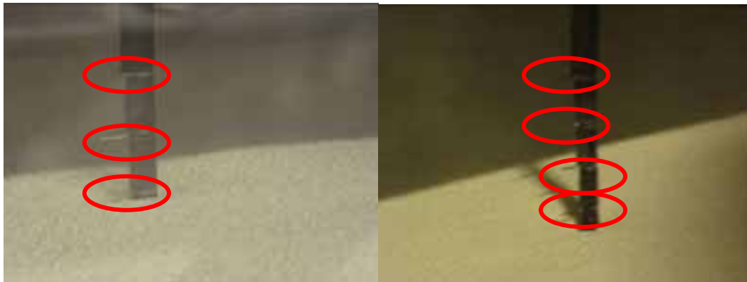
Figure 10 : Left: Height of the bed at the end of hydration reaction; - Right: Height of the bed at the end of dehydration reaction.
