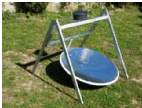
Fig. 1: Prototype of offset solar concentrator with a 80 cm diameter parabolic dish
