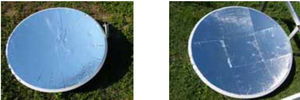
Fig. 7: Different types of reflective cover: polypropylene film (triangular pieces) and aluminium foil (square pieces)
