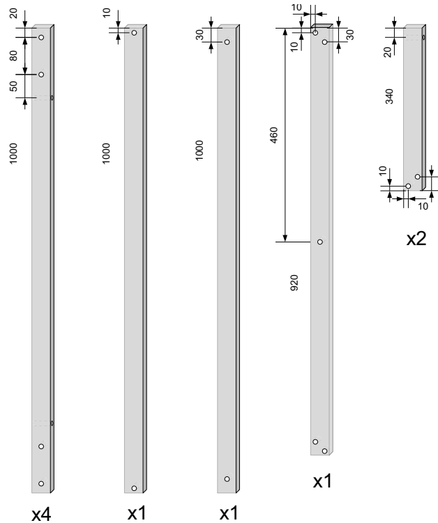
Fig. 16: Solar cooker parts and dimensions
