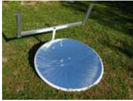
Fig. 12: U-shaped structure and parabola assembly
