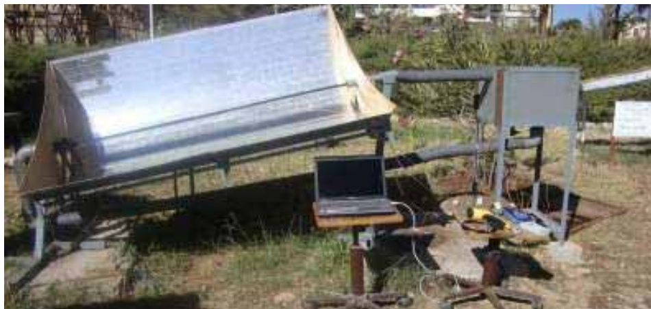
Figure 1: The solar cooker installed at the solar center of the Department of Mechanical Engineering
