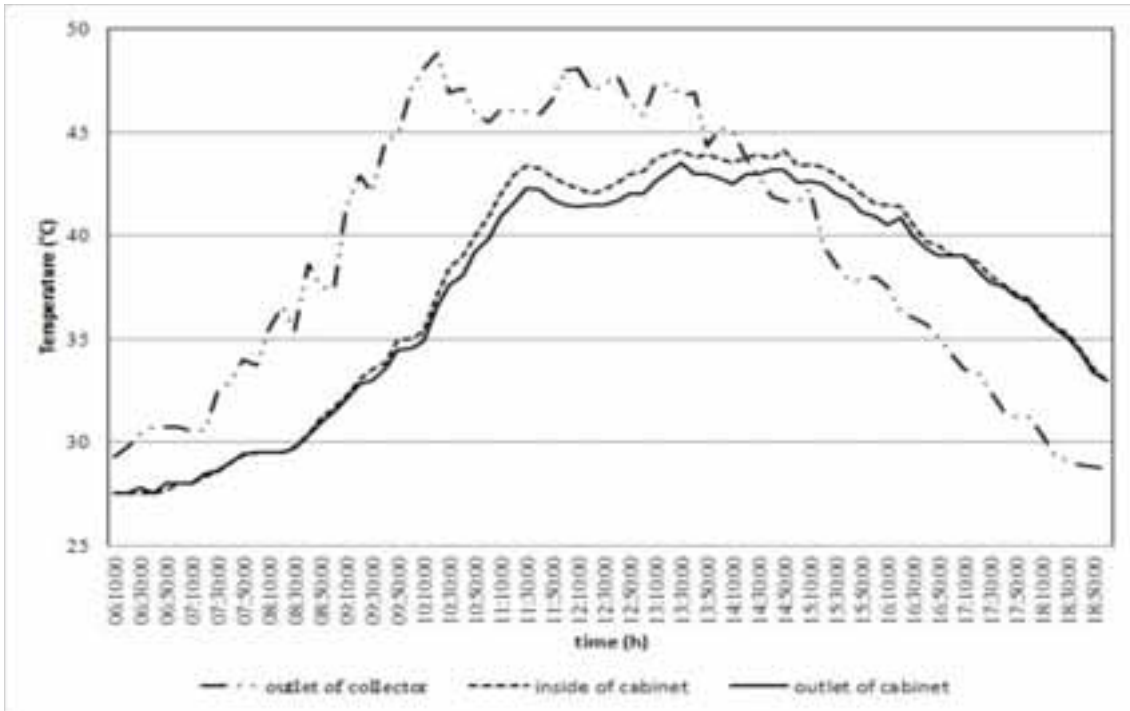
Fig. 3: Solar dryer temperature distribution at March 16 th 2011.
