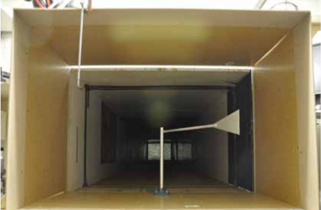
Fig. 3: A delta tail fin in the mid-section of the wind tunnel
