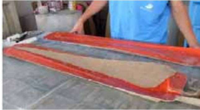
Fig. 1: Tissue cut according to the size of the inner mold
