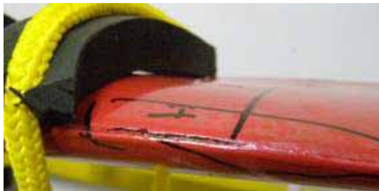
Fig. 11: Failure in test blade 2
