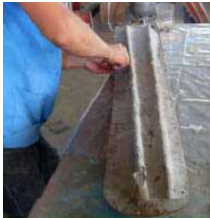
Fig. 5: The mold is closed
