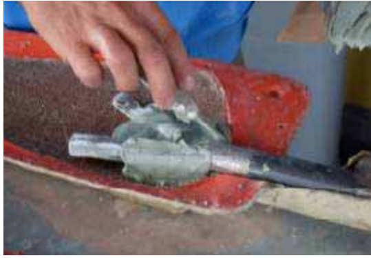
Fig. 4: Resin used to bind the metallic insert
