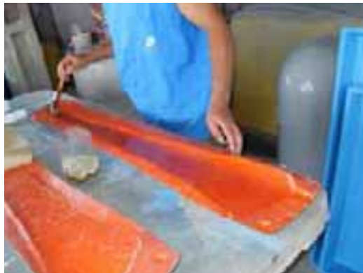
Fig. 2: Gel coat being applied on the mold surface
