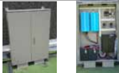
Fig 4: Chassis of HyPV for MCU, inverter and battery etc.
