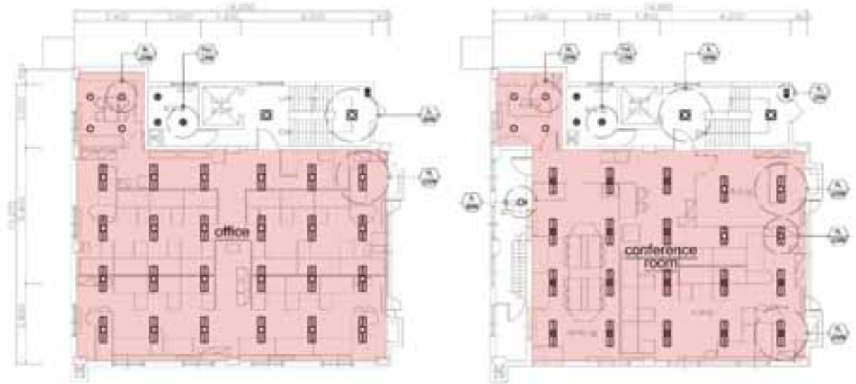
Fig. 3: office floor plan for sub-metering lighting energy use (L: 2~4F, R: 5F)
