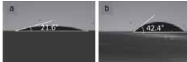
Figure 4: Contact angle of (a) DMSO and (b) formulated ink containing Cu-Zn-Sn-S precursor on Mo coated glass substrate.
