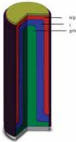
Fig. 1: The structure of nanowire solar cell
